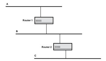
Notice that Router 1 can't forward the packet to segment C directly because it isn't directly connected to segment C. All Router 1 needs to know is that it should send packets destined for segment C to Router 2. Router 2 takes care of the rest. Similarly, if there was a segment D on the other end of segment C, Router 1 would still only need to know that the "next hop" toward that destination was Router 2.
